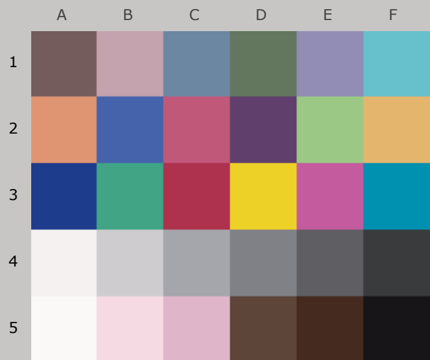
Colors after 240 Megalux-hours light exposure
