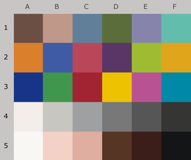
Colors after 50 Megalux-hours light exposure
