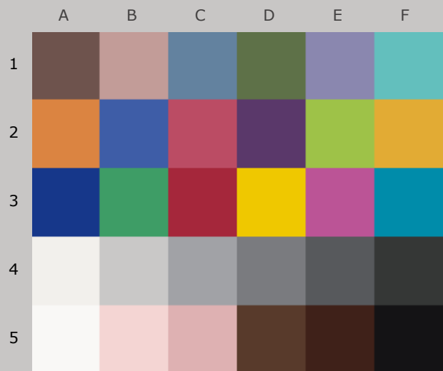
Colors after 120 Megalux-hours light exposure
