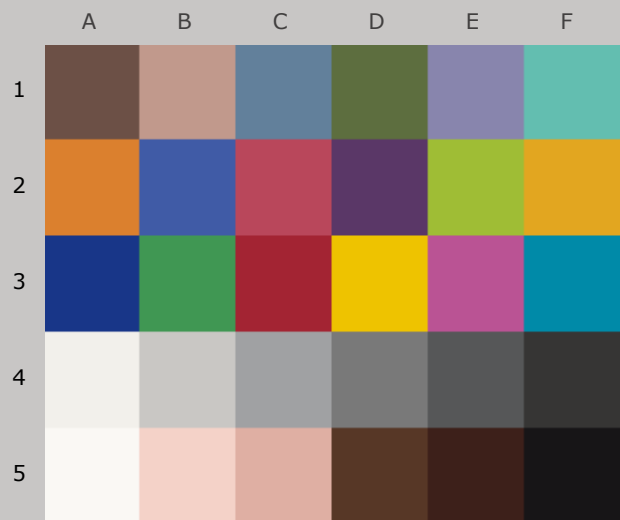
Colors after 60 Megalux-hours light exposure
