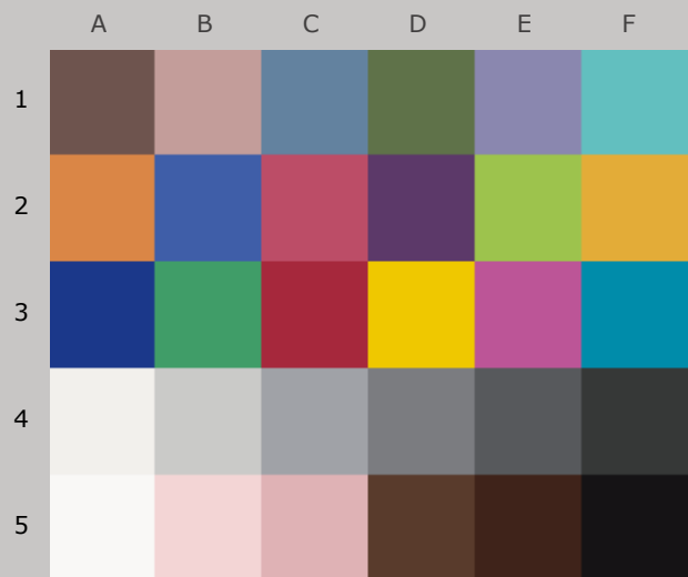
Colors after 130 Megalux-hours light exposure
