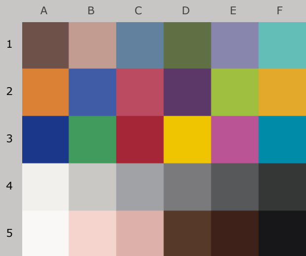
Colors after 90 Megalux-hours light exposure
