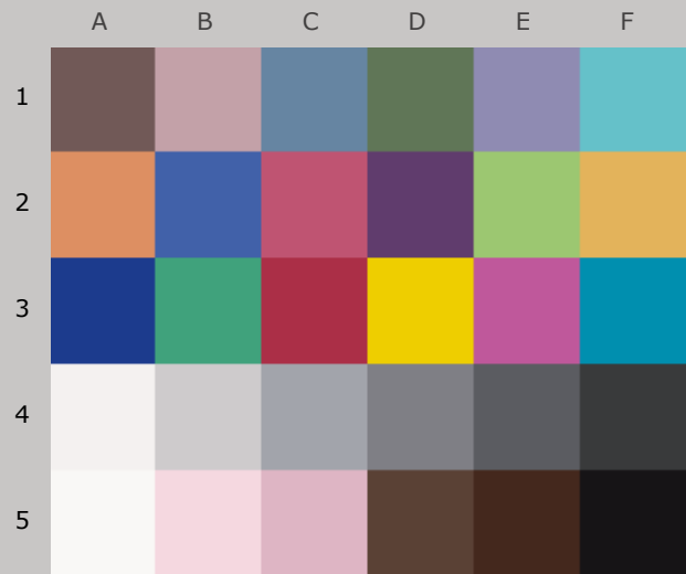
Colors after 200 Megalux-hours light exposure
