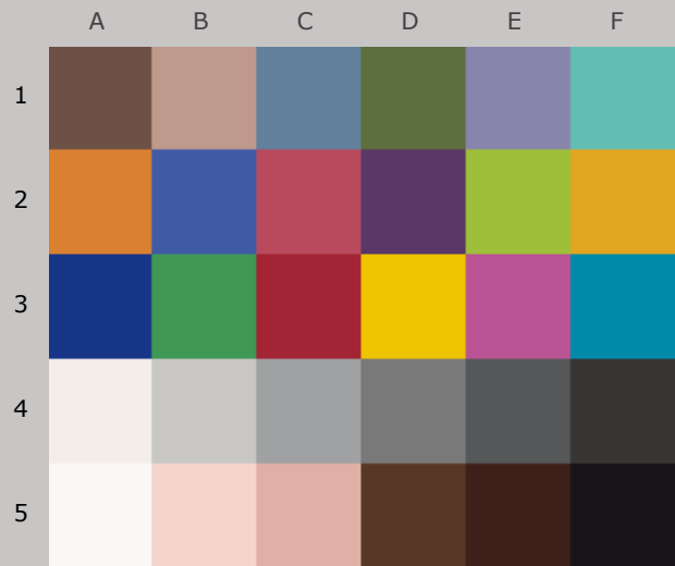
Colors after 70 Megalux-hours light exposure
