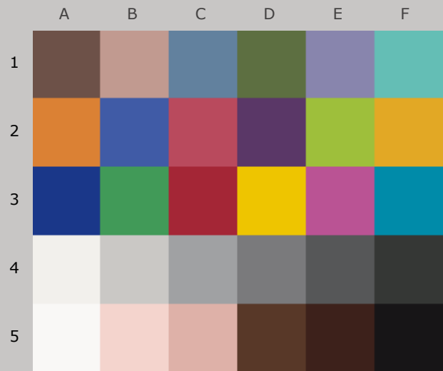
Colors after 80 Megalux-hours light exposure
