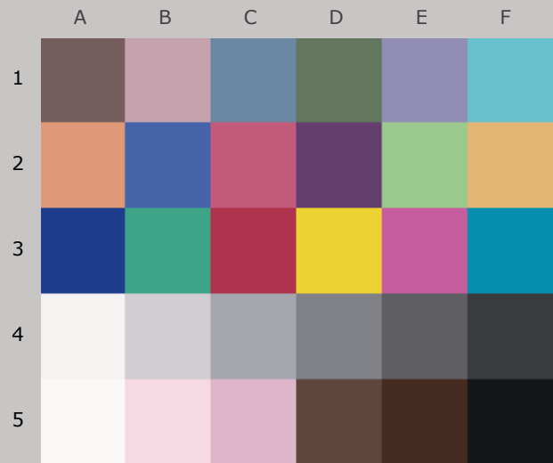
Colors after 260 Megalux-hours light exposure
