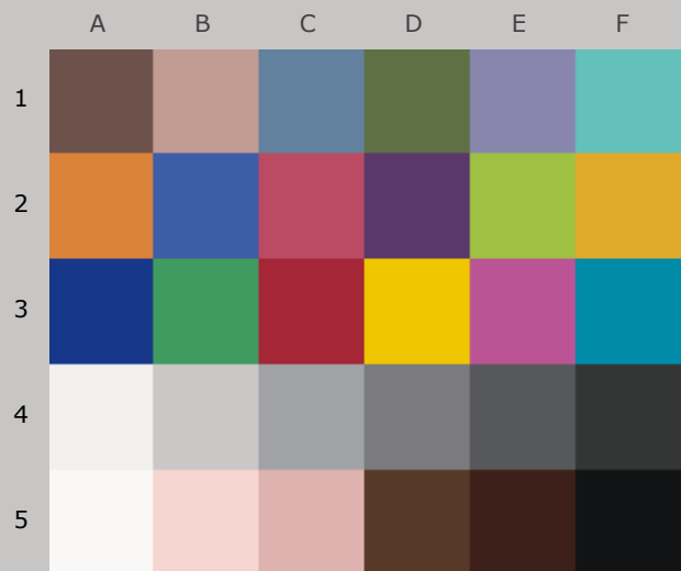
Colors after 100 Megalux-hours light exposure
