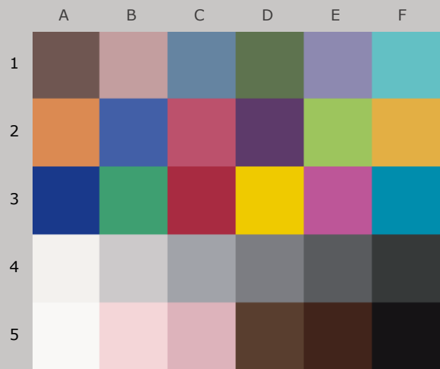
Colors after 160 Megalux-hours light exposure
