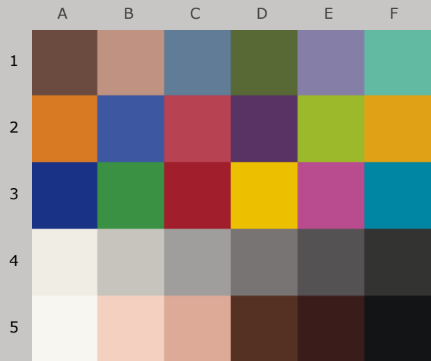
Colors at Zero Megalux-hours of Light Exposure (same as original print colors)
