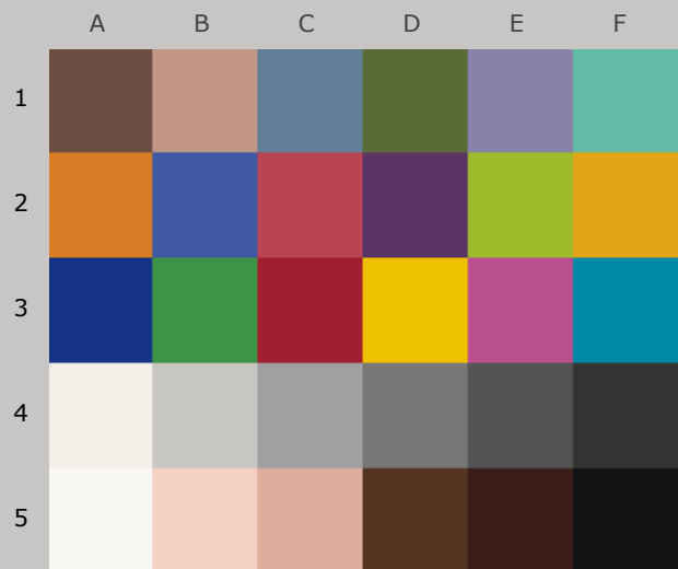
Colors after 20 Megalux-hours light exposure
