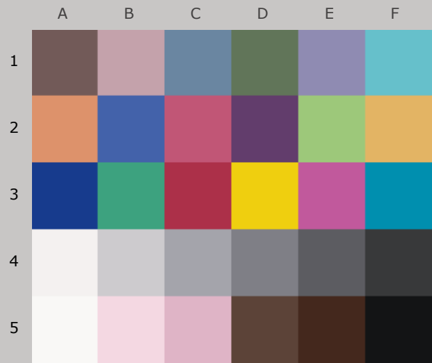
Colors after 220 Megalux-hours light exposure
