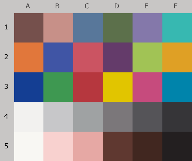
Colors after 80 Megalux-hours light exposure
