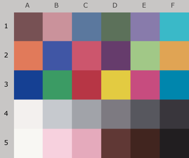
Colors after 180 Megalux-hours light exposure
