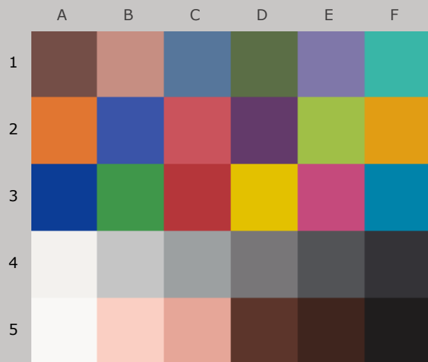
Colors after 20 Megalux-hours light exposure
