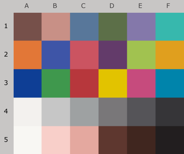
Colors after 60 Megalux-hours light exposure
