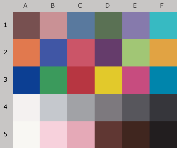
Colors after 150 Megalux-hours light exposure
