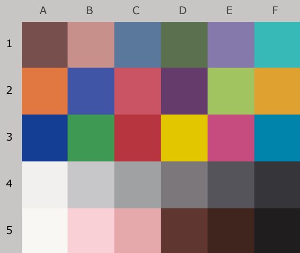
Colors after 110 Megalux-hours light exposure
