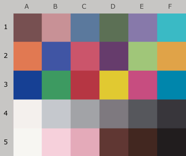
Colors after 160 Megalux-hours light exposure
