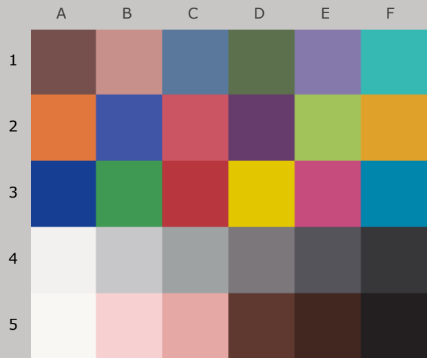
Colors after 90 Megalux-hours light exposure
