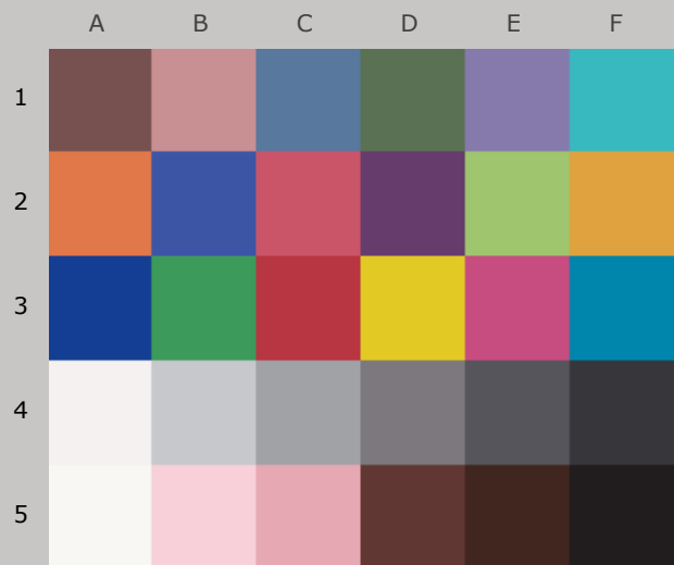
Colors after 140 Megalux-hours light exposure
