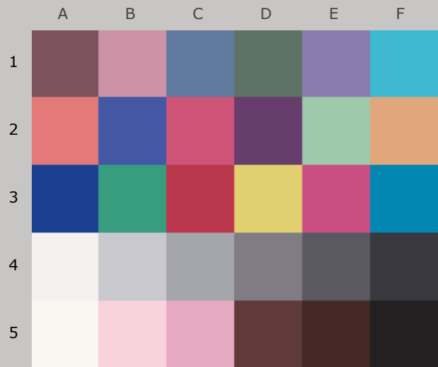
Colors after 260 Megalux-hours light exposure
