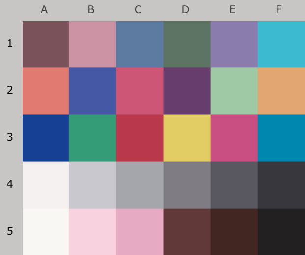
Colors after 240 Megalux-hours light exposure
