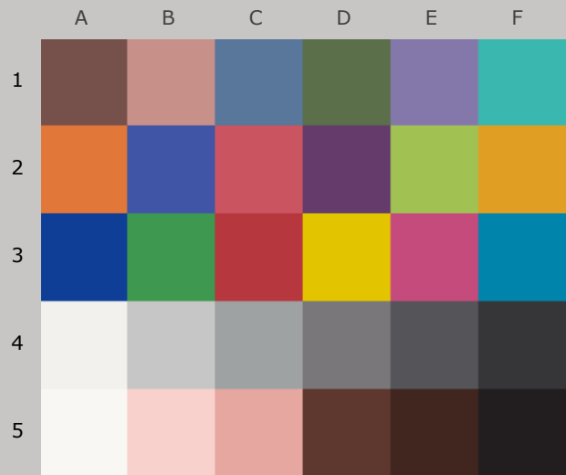
Colors after 70 Megalux-hours light exposure
