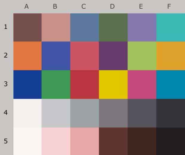
Colors after 100 Megalux-hours light exposure
