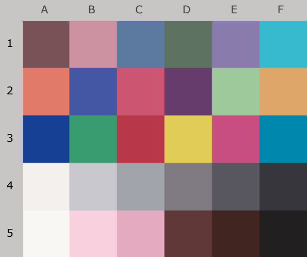
Colors after 220 Megalux-hours light exposure
