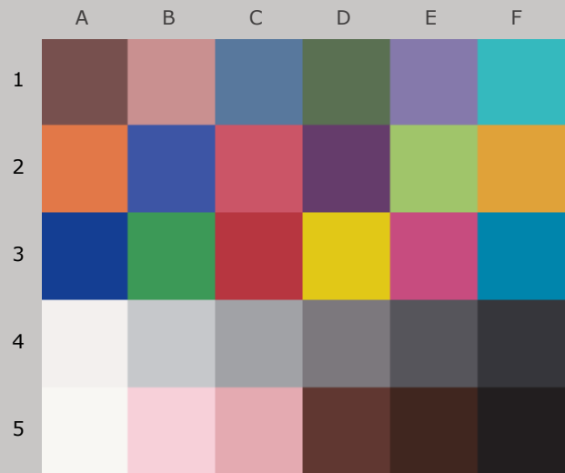
Colors after 130 Megalux-hours light exposure
