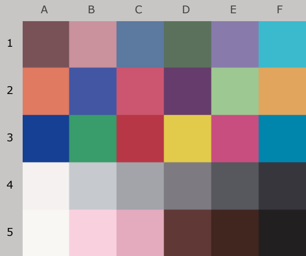
Colors after 200 Megalux-hours light exposure
