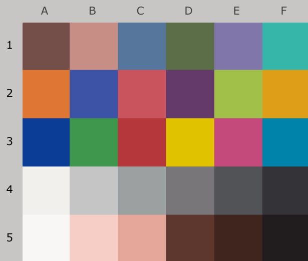
Colors after 40 Megalux-hours light exposure
