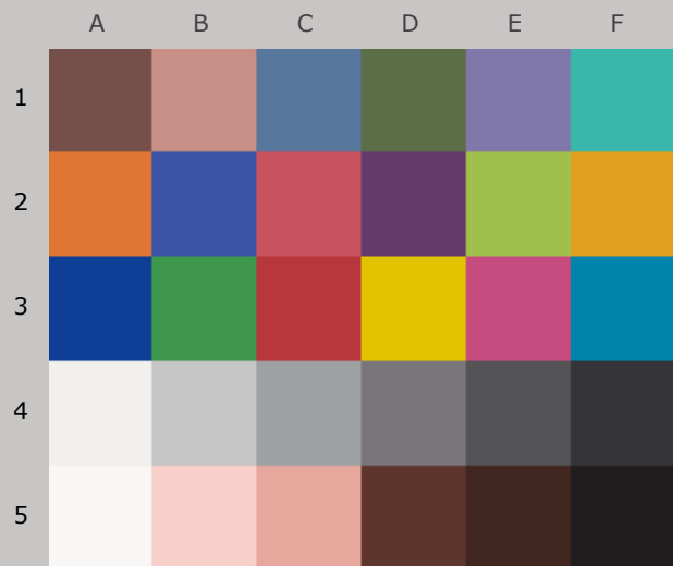
Colors after 50 Megalux-hours light exposure
