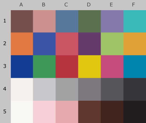
Colors after 120 Megalux-hours light exposure
