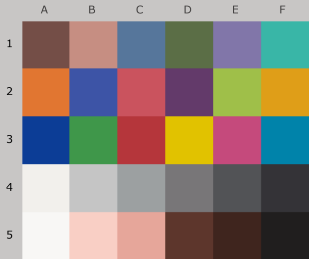
Colors after 30 Megalux-hours light exposure
