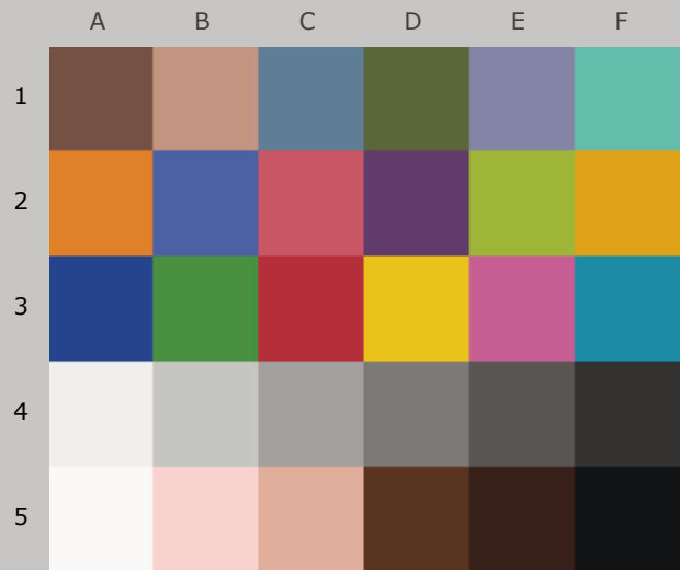
Colors after 60 Megalux-hours light exposure
