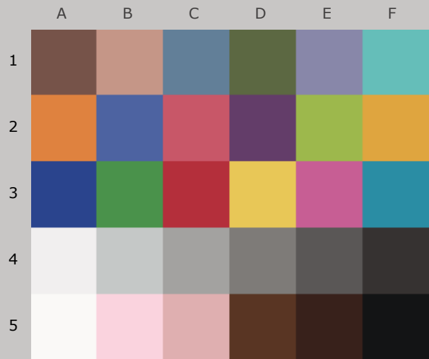
Colors after 120 Megalux-hours light exposure
