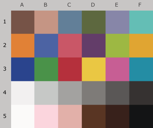
Colors after 100 Megalux-hours light exposure
