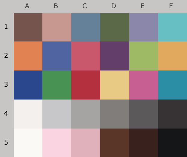
Colors after 160 Megalux-hours light exposure
