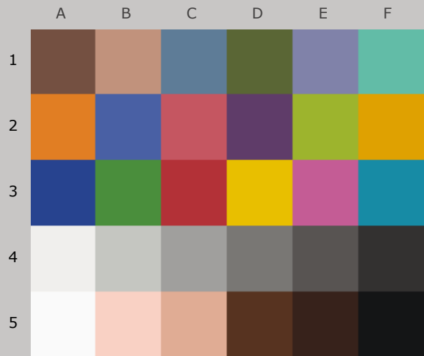
Colors after 20 Megalux-hours light exposure
