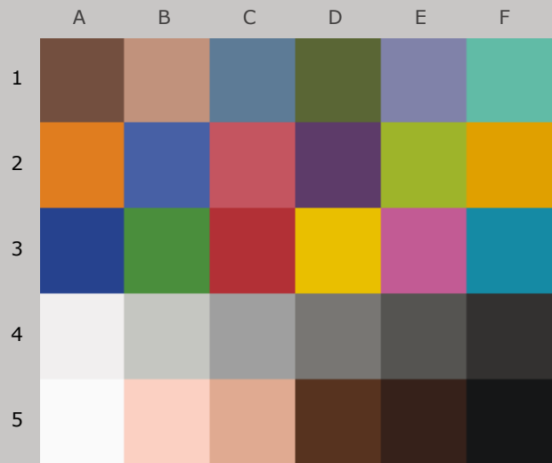
Colors after 10 Megalux-hours light exposure
