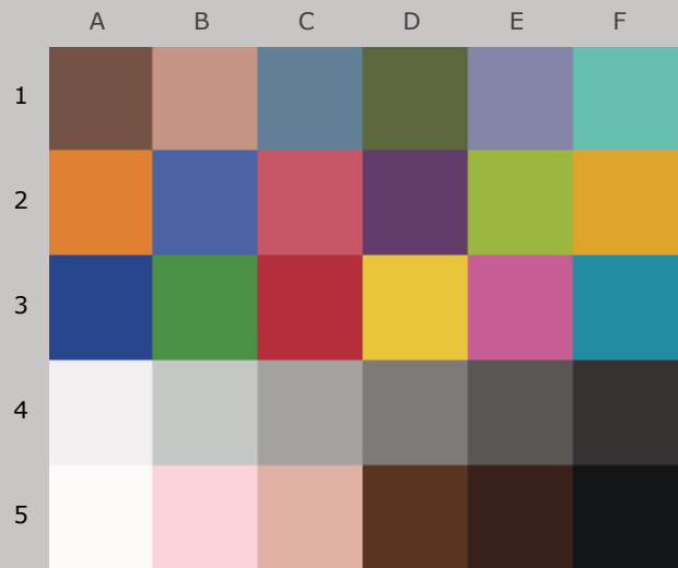
Colors after 90 Megalux-hours light exposure
