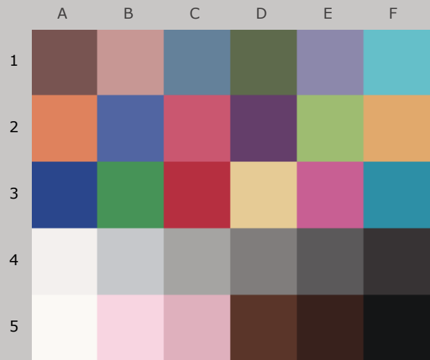
Colors after 180 Megalux-hours light exposure
