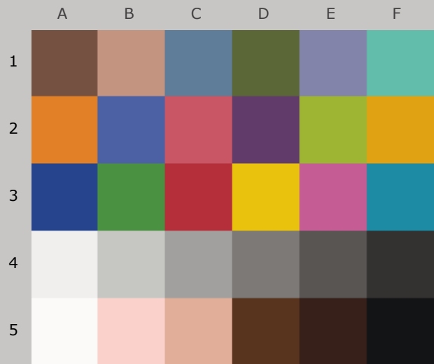
Colors after 50 Megalux-hours light exposure
