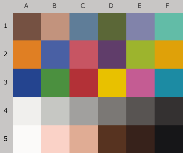
Colors after 30 Megalux-hours light exposure
