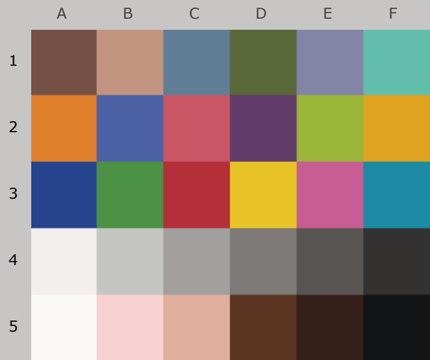
Colors after 70 Megalux-hours light exposure
