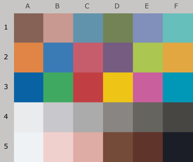
Colors after 70 Megalux-hours light exposure
