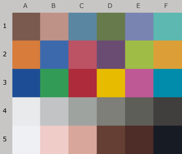
Colors after 20 Megalux-hours light exposure
