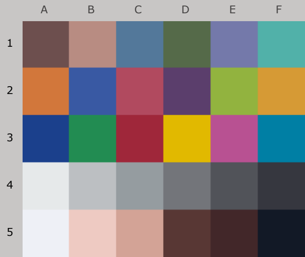
Colors at Zero Megalux-hours of Light Exposure (same as original print colors)
