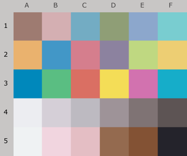
Colors after 220 Megalux-hours light exposure
