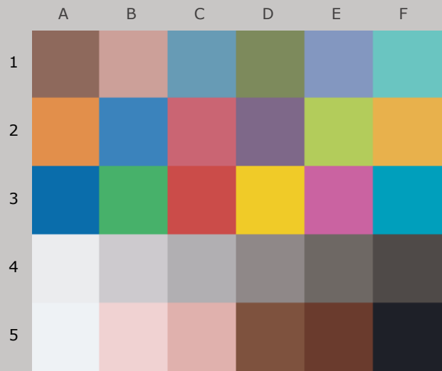
Colors after 110 Megalux-hours light exposure
