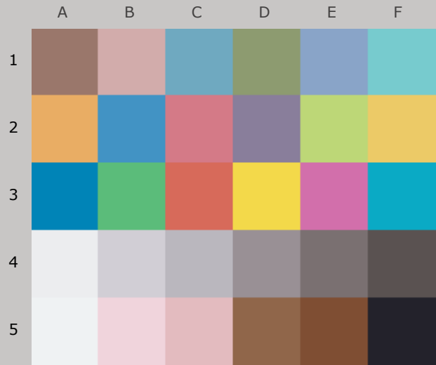
Colors after 200 Megalux-hours light exposure
