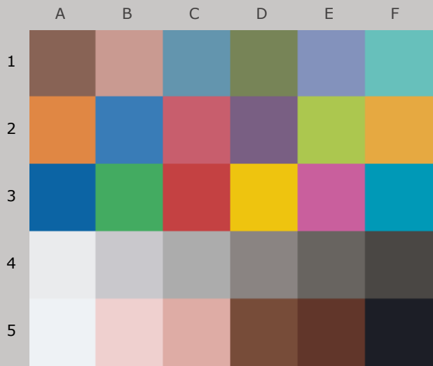
Colors after 80 Megalux-hours light exposure
