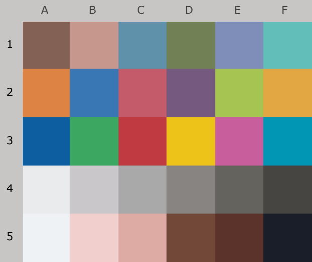
Colors after 60 Megalux-hours light exposure
