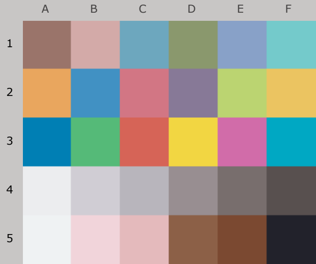
Colors after 180 Megalux-hours light exposure
